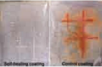
Self-healing coating (left) and control coating (right) after 24-hour immersion in salt water
